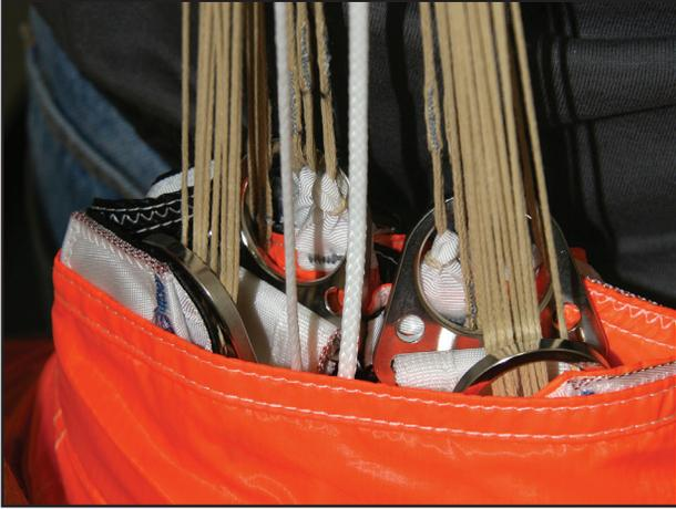
This photo shows a detailed view of the ring orientation and lanyard position before the tail is wrapped tightly above the rings; as illustrated in the following photo.
