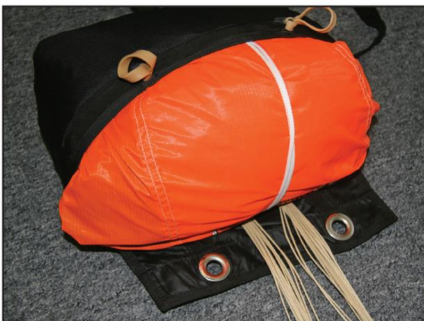
After the canopy is in the bag and the lanyard is in position securely, the pack job can be completed as normal with the stowing of the lines.
