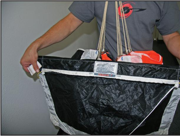
Orient the slider for ring attachment such that the warning label is readable. The white tape should be facing away with the lanyard coming off the trailing edge running freely towards the tail of the canopy.
