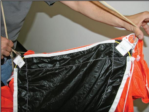
Repeat this process by continuing counter clockwise along the slider edge to the next corner, assembling the ring corners as you go until you've secured all four corners.
