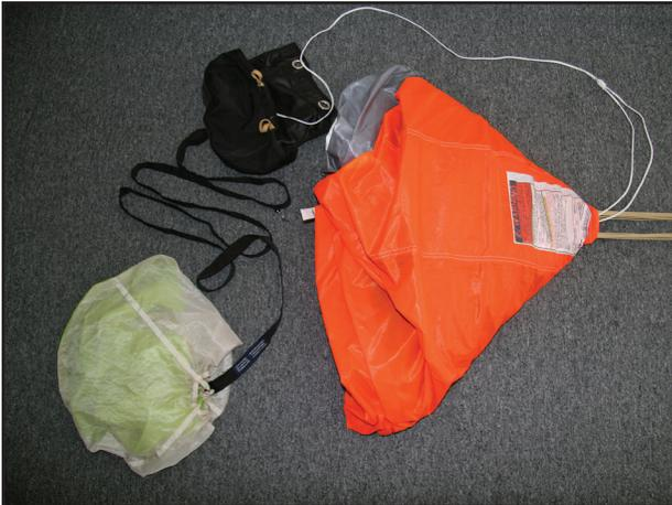
After the tail is wrapped, lay the canopy down on the ground with the RDS lanyard and the bag draped loosely to the right as shown here.
