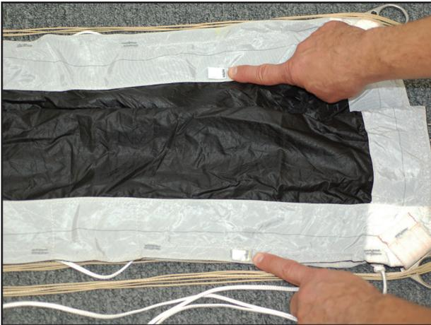
On the slider, you'll find four snaps on small tape tabs that will mate with the snaps on the canopy. Pictured are the right side leading edge and trailing edge snaps. (The trailing edge of the slider is identified by the RDS lanyard)
