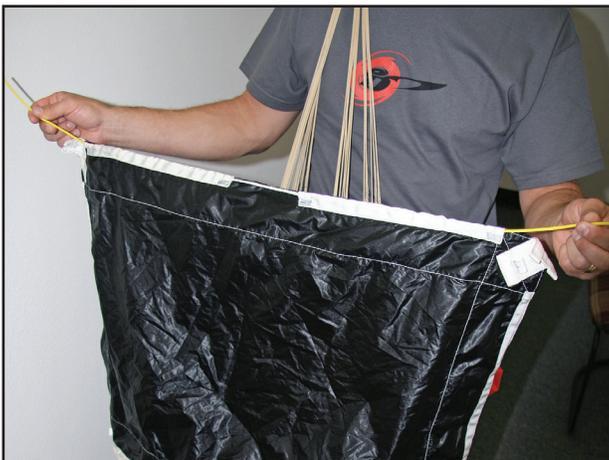
NOTE: Be sure that the release line is taut with no twists between the gap in the sleeves, removing any excess slack.
