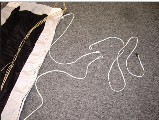
Next, remove the longer length of line in the lanyard assembly by undoing the larks head at the point where the lanyard junctions into two lines.
