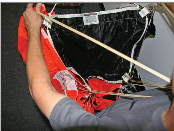
Upon complete assembly of all corners, perform a continuity check of the slider by raising the trailing edge up to show all rings and visually tracing your eyes from corner to corner. Check for proper ring and slider orientation.
