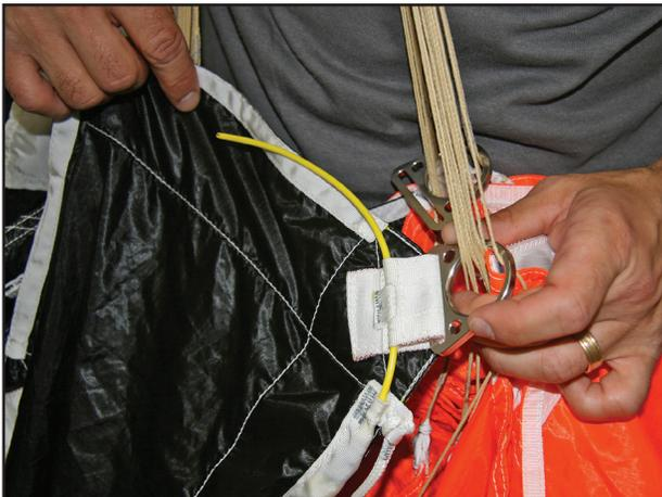
Route the yellow release cable thru all three loops. Make sure not to skip any of the loops in this process.
