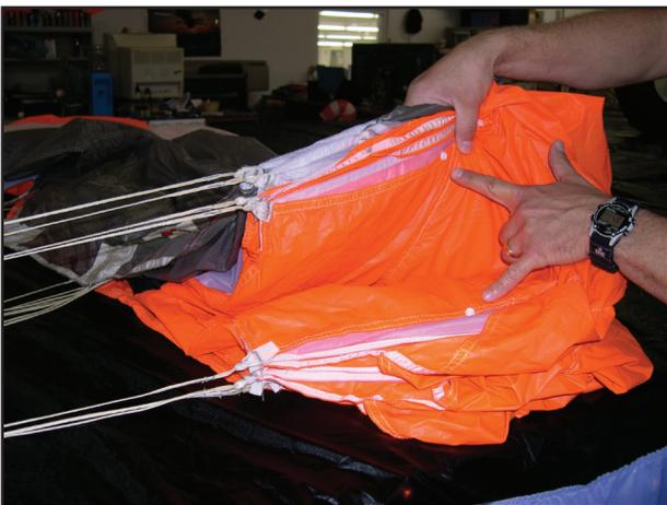
This canopy is equipped with plastic snaps that help secure the slider to the canopy during packing. Two snaps are located on the leading edge tape of the center cell.
