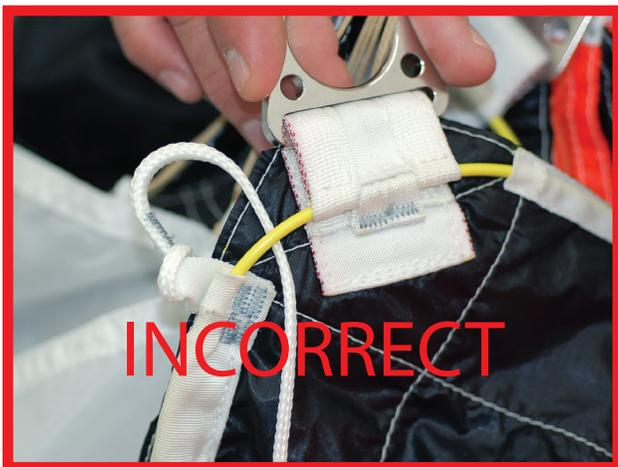
*CAUTION!! DO NOT ALLOW THE LANYARD TO GET TRAPPED UNDER THE YELLOW CABLE. The photo to the left shows an incorrect routing.*
