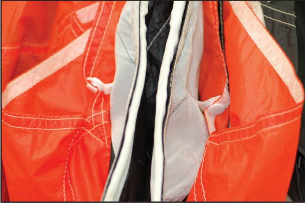
Fasten the leading edge slider snaps onto the canopy's leading edge center cell snaps.
