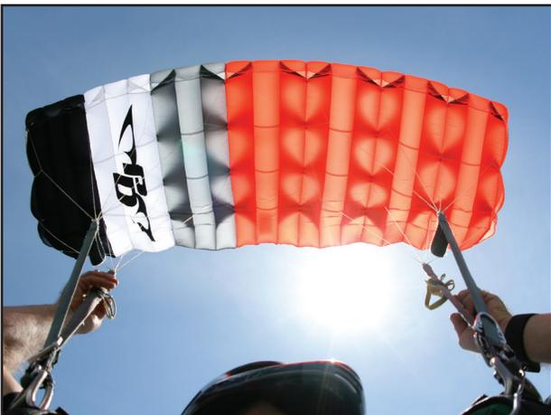
Before releasing your toggles, make sure that all four rings have been pulled down to the bottom of the risers.
