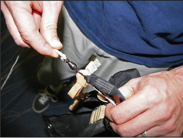
Attach the swivel at the end of the lanyard assembly to the deployment bag using a Slink or Mini-link. Larks head a spare rubber band around the attachment in order to stow the excess lanyard later during packing.
